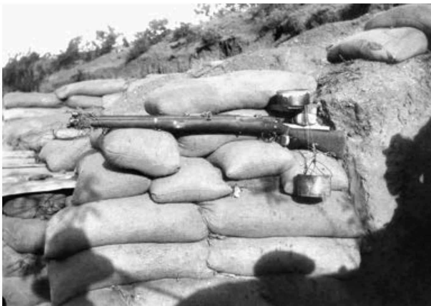
AWM G01291. Gallipoli Peninsula, 17 December 1915. A delayed action device for firing a rifle by means of weights operated through water escaping from one tin into another. A rifle could be left to operate twenty minutes after the device was set. Six rifles were left by 3rd Brigade to fire following the departure of the last party
